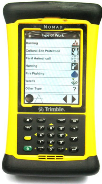
Figure 4. The Trimble Nomad TDS800LC unit on which the Djelk Rangers run CyberTracker showing the operational screen for the Djelk Land Ranger Data Application. (Photo © J. Koenig.)
